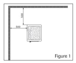
2. The safety distance stated in section 1 (500 mm) can be reduced by half to 250 mm if so-called light, single-layer thermal protection is installed. A single-layer, light thermal shield can be made from min. 7 mm thick fire-resistant fibre-reinforced cement board or from min. 1 mm thick metal sheet which has been fixed sufficiently tightly to the wall. A ventilation gap of 30 mm must be left between the thermal shield and the wooden surface, e.g. using pipe sleeves. (Figure 2)
