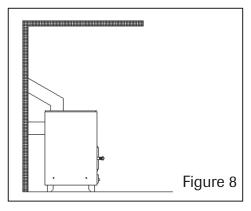
Do not install the flue adapter pipe too deeply into the chimney flue, as this will reduce the flue draw. The gap between the flue adapter pipe and the chimney flue must be insulated e.g. with mineral wool.
