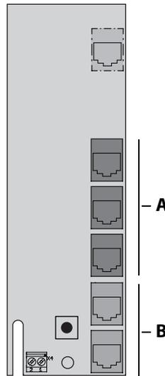
**A** RJ10 plug for sensor line
