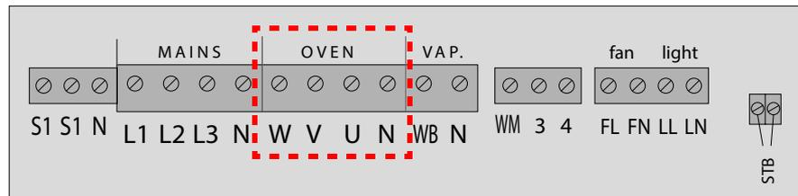
The switching output of the control unit for the sauna heater has a max. of 9 kW resistive load. It can be expanded as needed by an optional output controller (LSG) so that it is possible to connect sauna heaters with an output greater than 9 kW.
